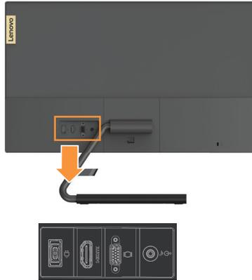
3. Connect one end of the HDMI cable to the monitor HDMI connector and the other end to the computer.
