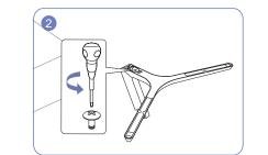
Turn the connecting screw at the bottom of the stand base to separate it.
