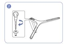
Insert the stand neck into the stand base in the direction shown in the figure. Check that the stand neck is firmly connected.
