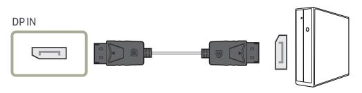
To display 3440 x 1440 @ 75 Hz, use a DP cable that supports 3440 x 1440 @ 75 Hz. Make sure that the graphics card of the DP source supports 3440 x 1440 @ 75 Hz.
