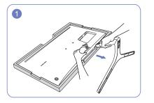
Place the protective Styrofoam (cushion) included in the package on the floor and place the product facing down on the Styrofoam, as shown in the image. If Styrofoam is unavailable, use a thick sitting mat. While holding the monitor with one hand, pull the stand neck with your other hand to in detach the stand as shown in the figure.
