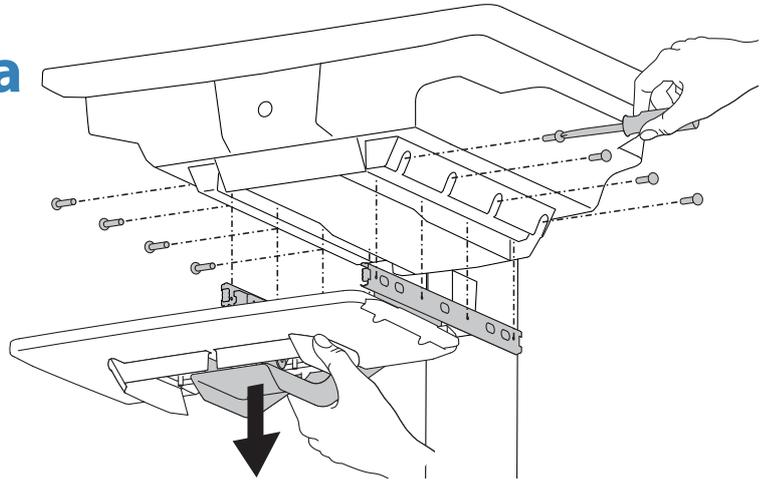
**NOTE:** Use a PH2 Phillips screwdriver to remove these screws. Some force may be required to remove these screws if red loctite is present.
