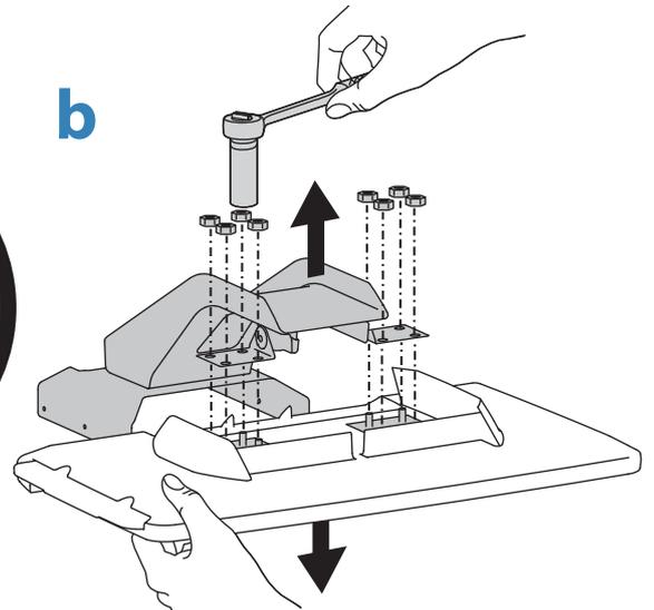
**5** Install keyboard tray onto height adjustable keyboard arm using 8 nuts.
