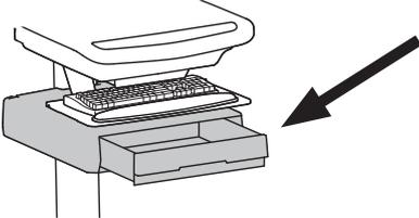
If there is a drawer on the cart, you'll need to adjust the keyboard arm to fit onto the cart.
