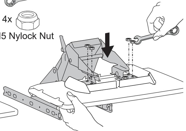
**6** Install height adjustable keyboard arm with keyboard tray back onto the cart using 8 Phillips screws.
