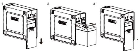
1. Slide off the battery cover at the back of the DTC36U12V unit.
