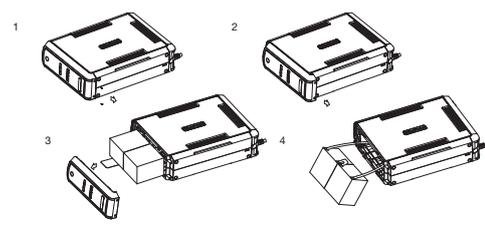
1. Turn the UPS on its side. Remove the front panel retaining screws located on the bottom of the UPS.
