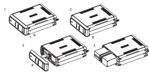
1. Turn the UPS on its side. Remove the front panel retaining screws located on the bottom of the UPS.
