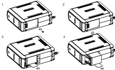
1. Turn the UPS on its side. Remove the retaining screw located on the bottom of the UPS.
