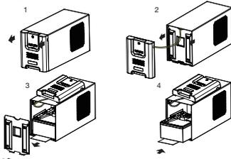
1. Remove the front panel of the UPS.
