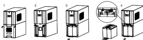
1. Remove the front panel of the UPS and two screws from the battery compartment cover and slide the cover completely off of the unit.
