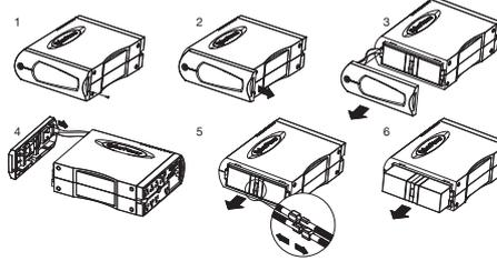
1. Place the UPS on its side to locate and remove the front panel retaining screws from the bottom of the UPS.
