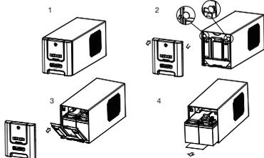
1. Remove the front panel of the UPS.
