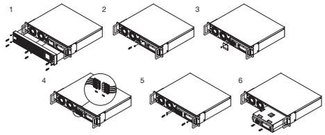
1. Remove the six retaining screws, and remove the front panel from the UPS.
