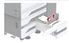
In tandem trays, pull out handle C, and then open the inner cover
