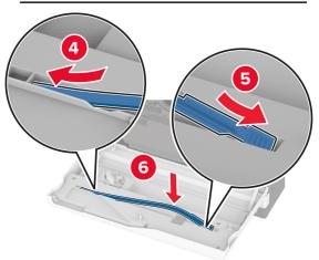
Insert the printhead wiper back into place.
