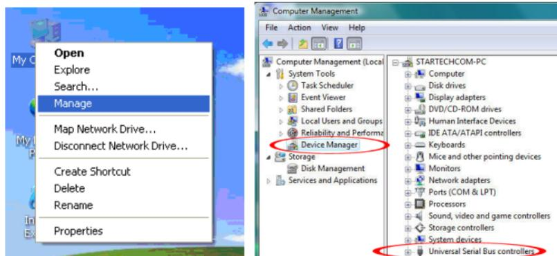
In the Device Manager, under the Universal Serial Bus Controllers category, you should see the new entries for the USB 3.0 controller card.
