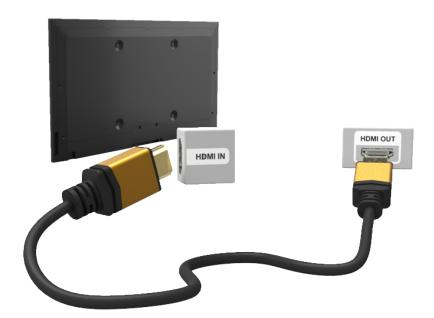
Once the connection has been made, press the **SOURCE** button to select the connected external device.
