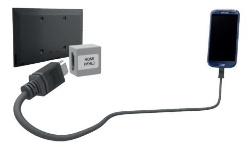
Once the connection has been made, press the **SOURCE** button to select the connected external device.
